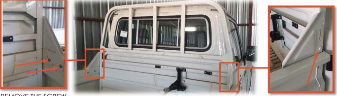
REMOVE THE SCREW WITH A PHILIPS SCREWDRIVER.
